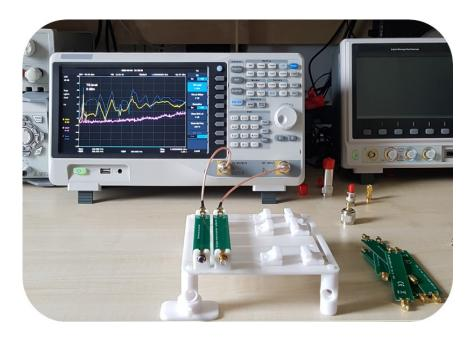
Figure 2: Test setup showing the PCB fixture details.
