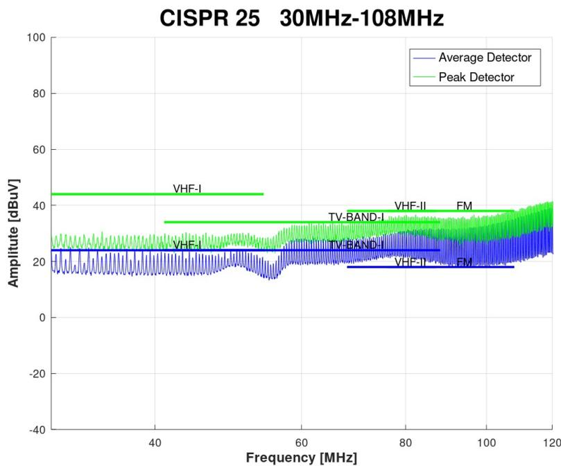
Figure 6: EMC conducted tests – DC-DC converter 30MHz-108MHz (without filter).
