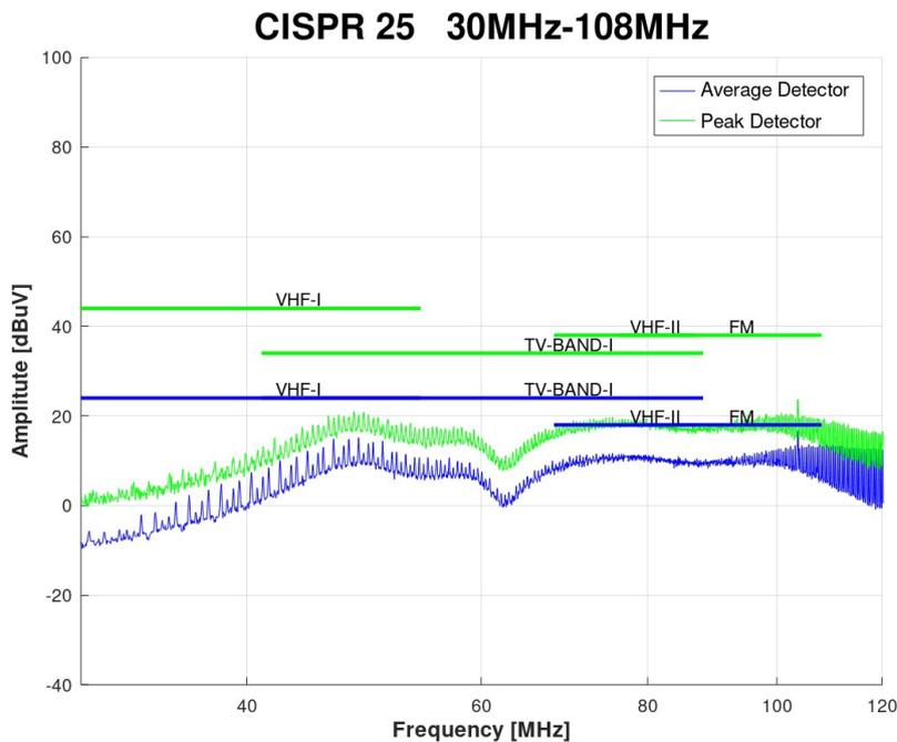
Figure 8: EMC conducted tests – DC-DC converter 30MHz-108MHz (with filter) .
