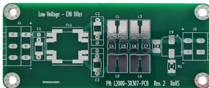
Figure 2: EMC filter PCB.
