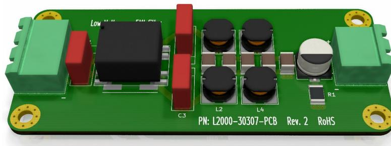
**Figure 3:** EMC filter assembled – using Wuerth common mode choke .
