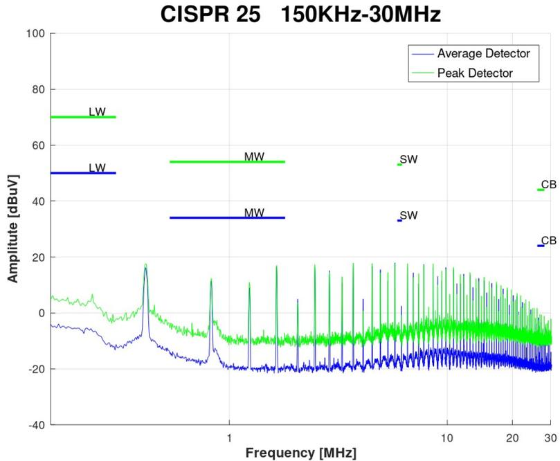
Figure 7: EMC conducted tests – DC-DC converter 150KHz-30MHz (with filter) .
