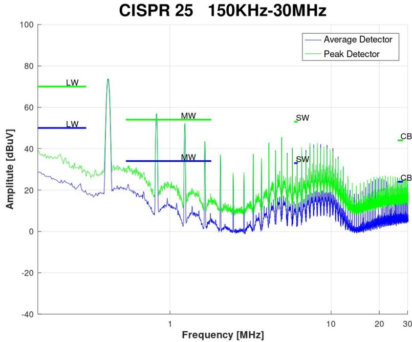
Figure 5: EMC conducted tests – DC-DC converter 150KHz-30MHz (without filter).
