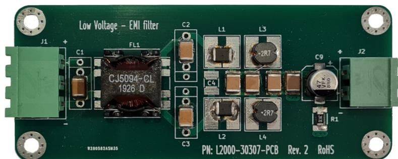
**Figure 4:** EMC filter PCB assembled with Coilcraft common mode choke.
